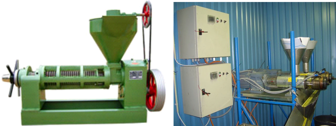
Figure 6 - Examples of oilseed presses: Zhengzhou 6YL-130 (LEFT) and two Taby 90's (RIGHT).
