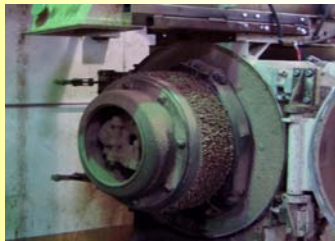
Pellets are extruded through 1/4" diameter die
