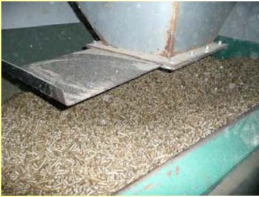
Pellets in the hopper bin after cooling
