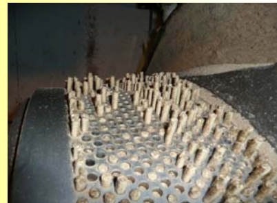
Exterior of the Extrusion Die
