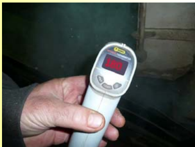
Mill operator checks the temperature of the pellets.
