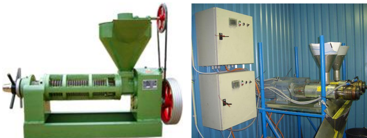
Figure 6 - Examples of oilseed presses: Zhengzhou 6YL-130 (LEFT) and two Täby 90's (RIGHT).
