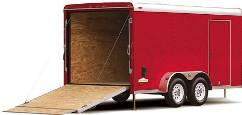
Figure 2 - Trailer Platform: Commercially available "landscaper's" trailer. Pace American Summit line, model SL714TA2, $6500 MSRP, 7.5' W x 14.5' L x 7' H, 4500 lbs payload.
