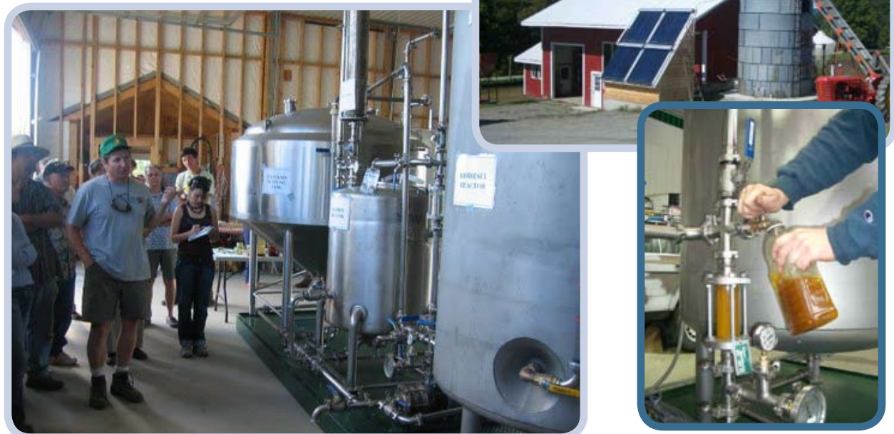
Clockwise from left: John Williamson describes biodiesel reactor during Field Day; solar grain dryer at State Line Biofuels; John takes a sample.
