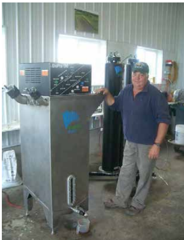
Roger Rainville (Alburgh) uses a 50-gallon Springboard Biodiesel BioPro 190 to make fuel at Borderview Farm.
