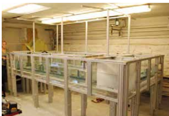
Overview of the flume filled with water. The lighting system suspended above the flume is not shown in this photo.
